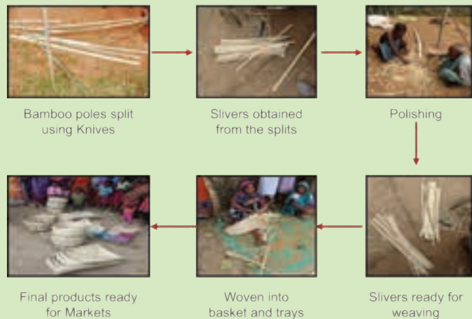
Figure 7: Production process for bamboo mats, baskets and trays
